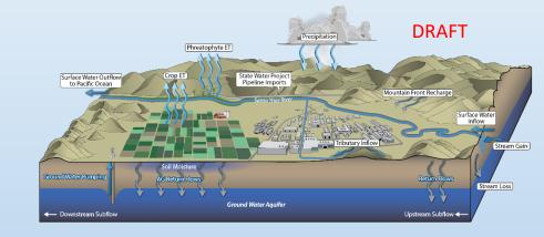
Hydrogeologic Conceptual Model 3D Geologic Visualization
