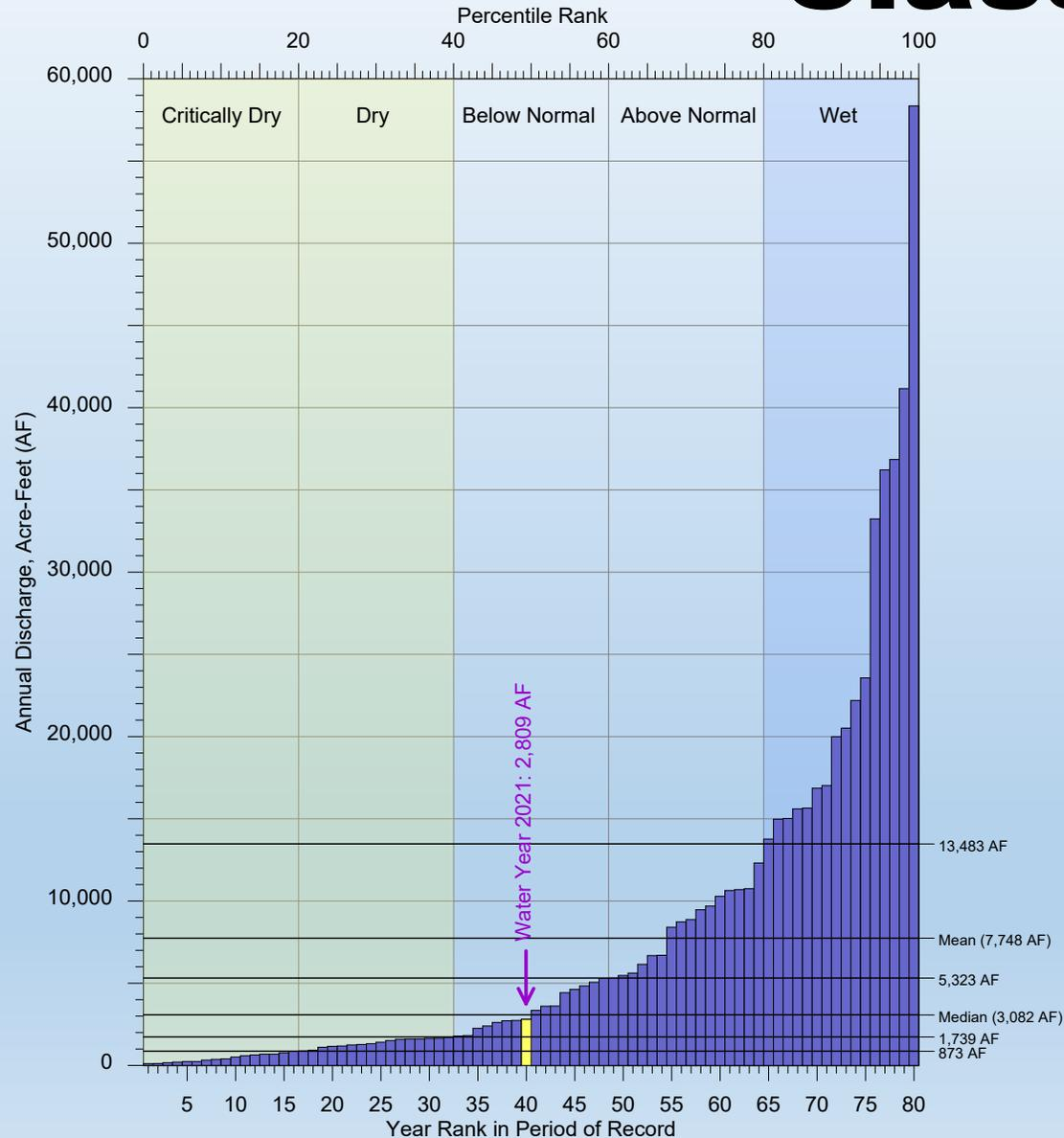
**Water Year 2021 Classified using same method as used in GSP, using Salispudes Creek USGS Streamflow Gage (11132500).**
