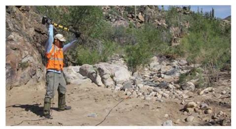
Seismic refraction surveying
